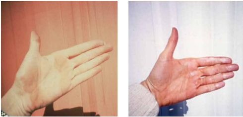
Failure in the Resin System Causes Chalking
